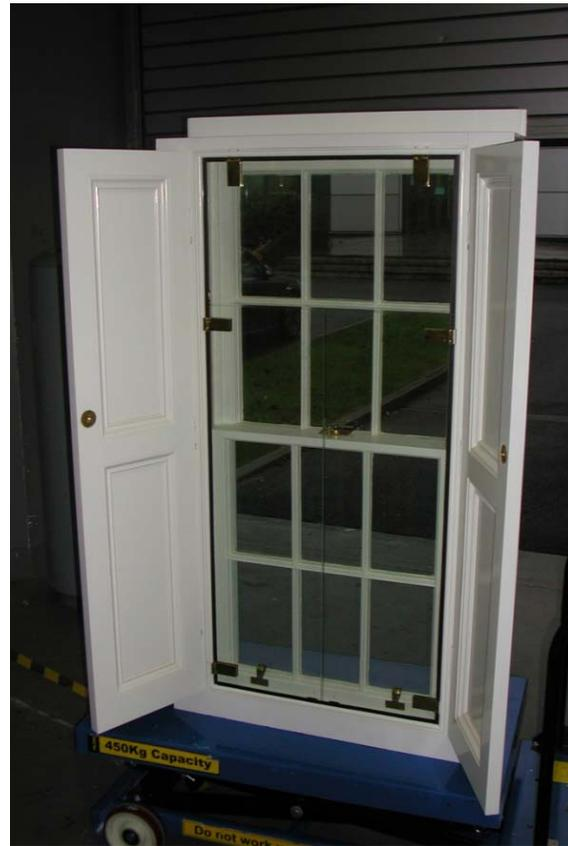
**Figure 2** Sliding sash window with glass and wooden shutters
