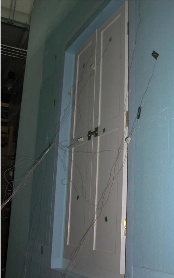
**Figure 11** Wooden shutter under test with temperature sensors attached
