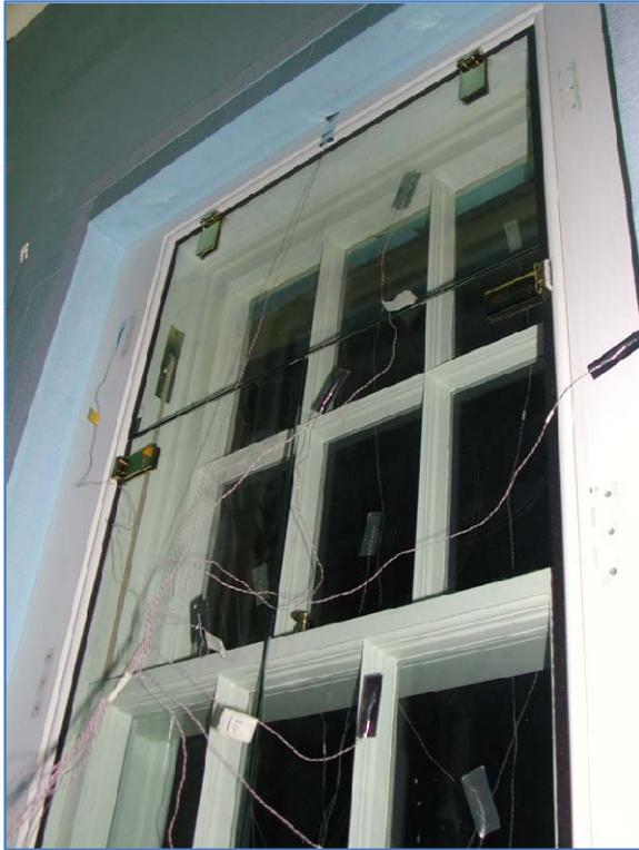
**Figure 9** Low-e glass shutters with sealing strip between shutters and frame
