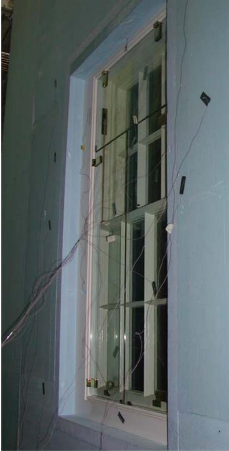
**Figure 7** Low-e glass shutters under test
