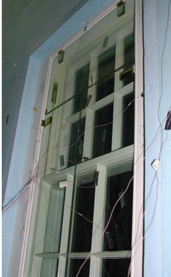
**Figure 8** Location of temperature sensors on the window under test
